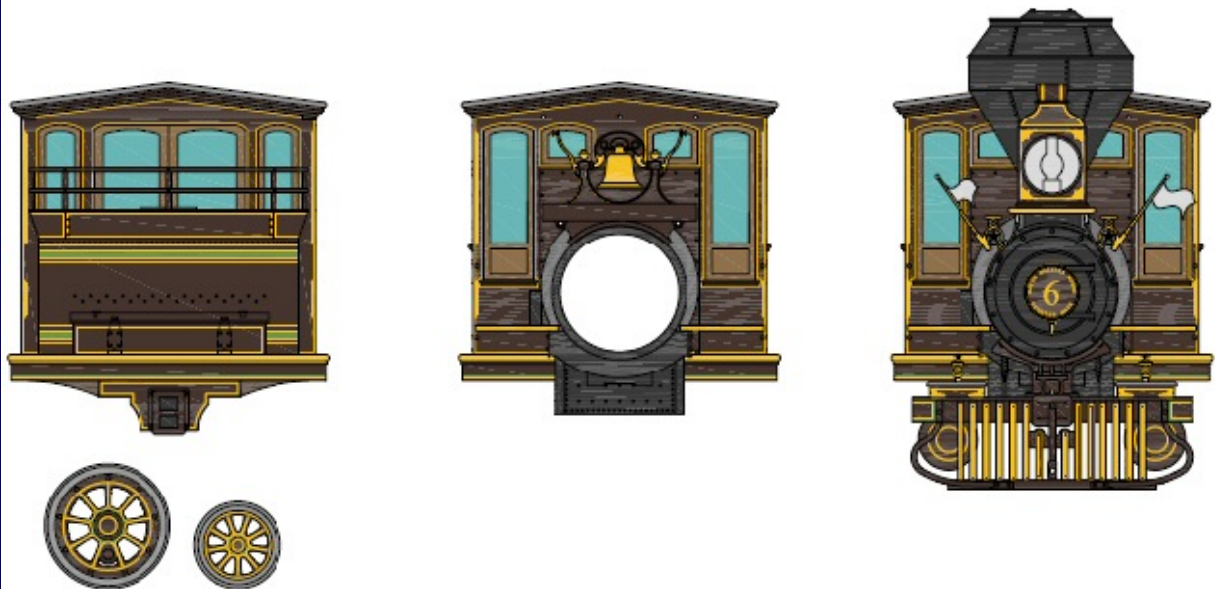
DENVER SOUTH PARK & PACIFIC RR MASON BOGIE #6 - 'TENMILE' 'AS BUILT' CONFIGURATION 1879
