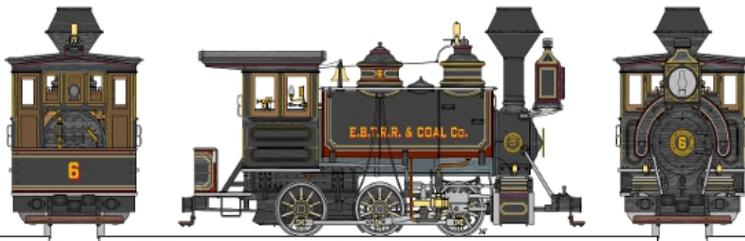
EAST BROAD TOP R.R. & COAL Co. 0-6-0ST #6 BALDWIN 6-22 D1, DRAWING 1 CONSTR No. 3733, 1875 BALDWIN PAINT STYLE: BLACK NO GOLD, EXCEPT ON WHEELS, STYLE 10
