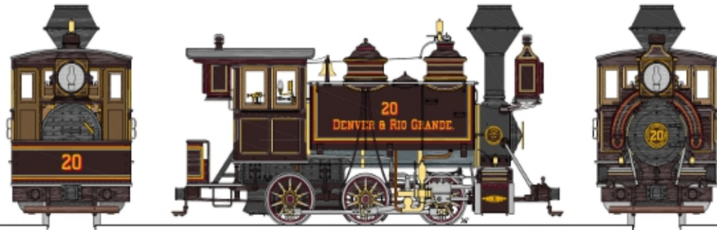
DENVER & RIO GRANDE Rwy CLASS 41 0-6-0ST #20 BALDWIN 6-22 D2, DRAWING 1 CONSTR No. 4067, 1877 BALDWIN PAINT STYLE: LARK & COLOR, STYLE 4 100 CUBIC FEET. DRAWINGS BELONGING TO DENVER & RIO GRANDE R.R. CO., DENVER, COLO., U.S.A. SPECIAL THANKS TO RICHARD POCKETT FOR BEARING MATERIAL
