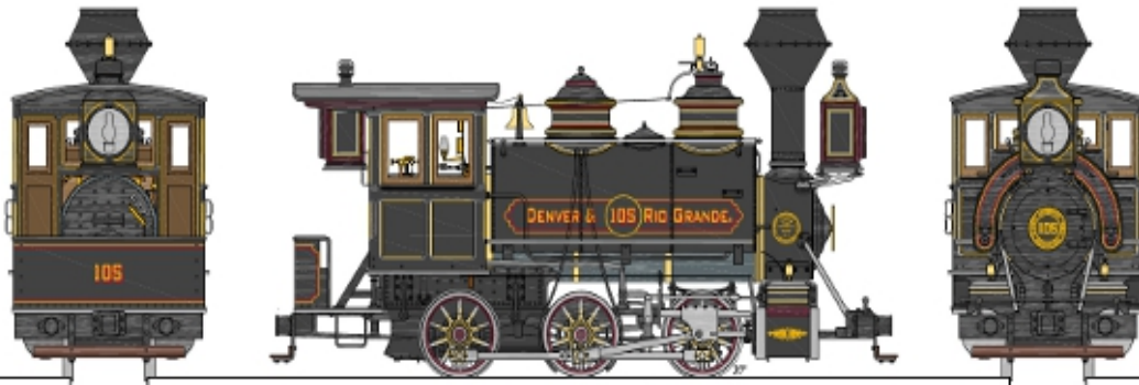
1881 - BLACK & COLOR, STYLE 98 DENVER & RIO GRANDE RMY CLASS 41 04-05T #105 BALDWIN 6-22 DS, DRAWING 1 CONSTR No. 573, 1881
